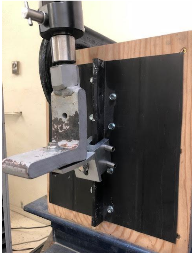
Figure B2b. Typical Failure Mode
