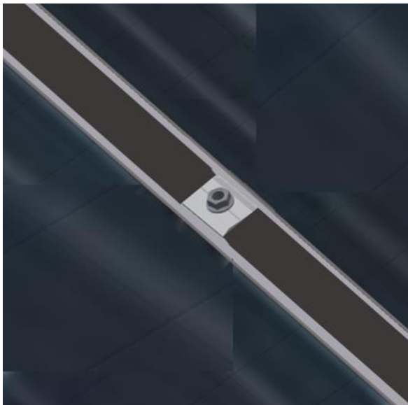
Install the EPDM Gasket leaving a 1/4 inch gap at the ends of the gasket.
